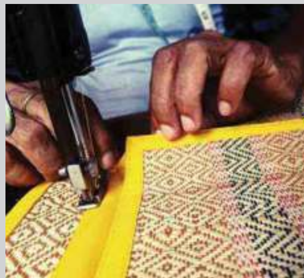
Stitching borders on the mats to ensure a neat finish to the product
