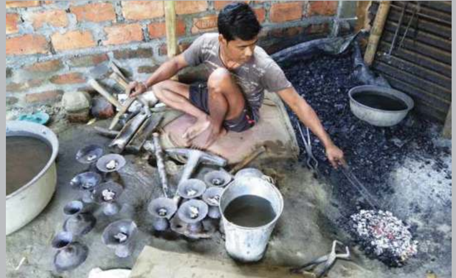
Making the bell-metal pliable by heating in an open furnace
